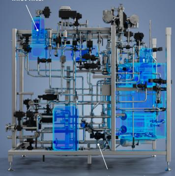
Condensate and waste water collector
